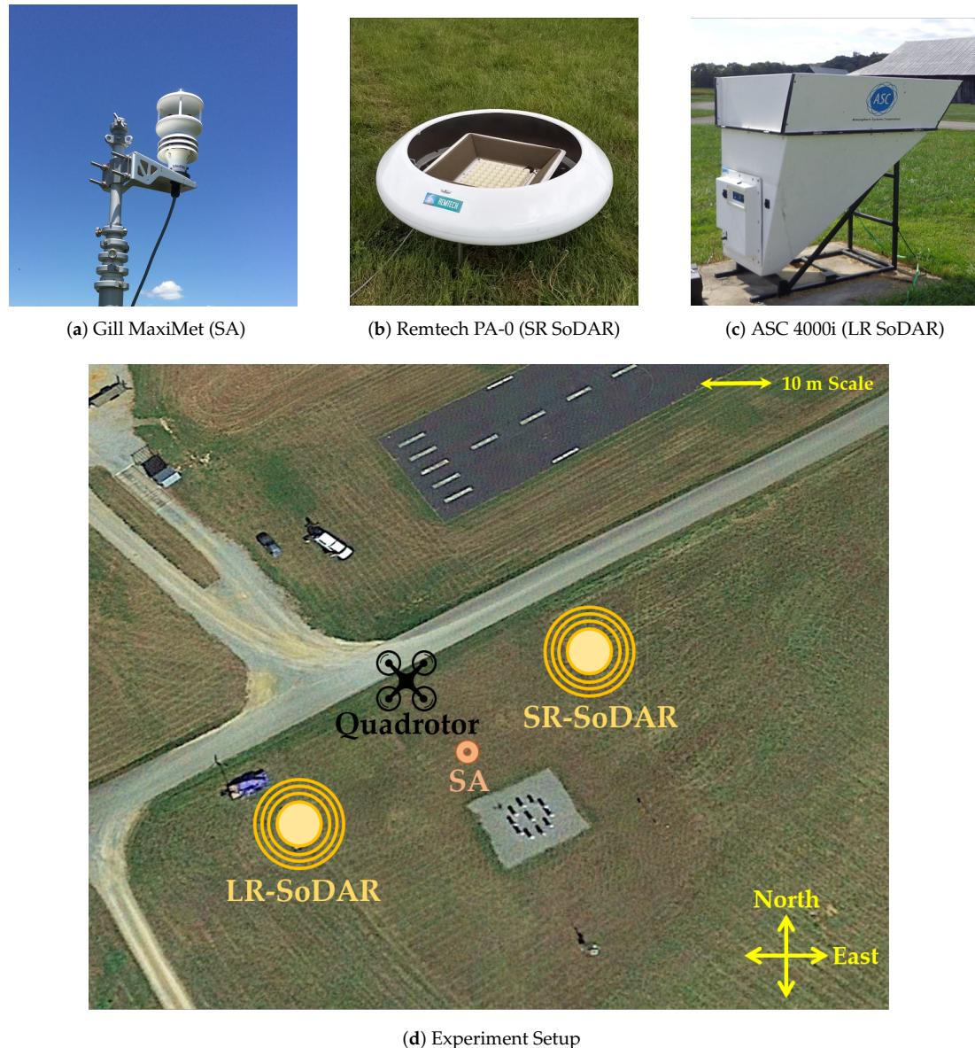
**Figure 4.** (a) The Gill MaxiMet sonic anemometer used to measure wind velocity 10 m AGL. (b) The Remtech PA-0 sensor (SR SoDAR) used to measure wind velocity from 10 to 120 m AGL. (c) The ASC 4000i sensor (LR SoDAR) used to measure wind velocity from 30 to 120 m AGL. (d) The experiment setup used to validate quadrotor wind estimates from 10 to 120 m AGL.
