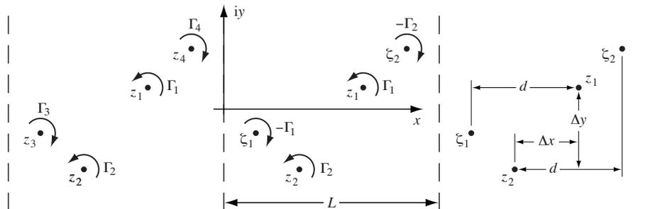
Figure 2: Model 2P configuration with two pairs of vortices per period.
