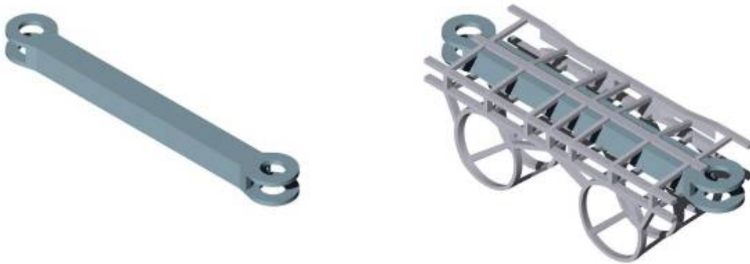
Figure 6.32: Wing carry through box: (a) standing alone and (b) integrated into surrounding bulkhead and longerons
