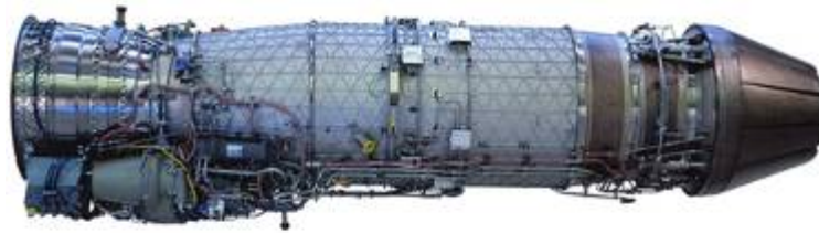
Figure 5.21: Rolls Royce EJ200 Low bypass ratio engine with afterburner 11
