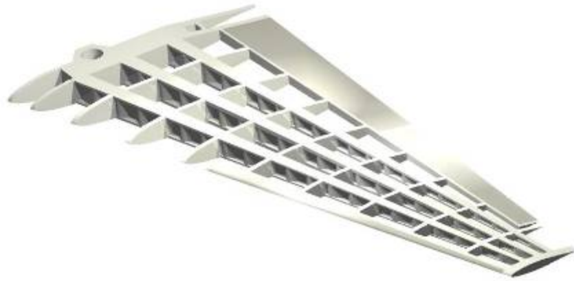
Figure 6.35: Wing structure with sine wave beams
