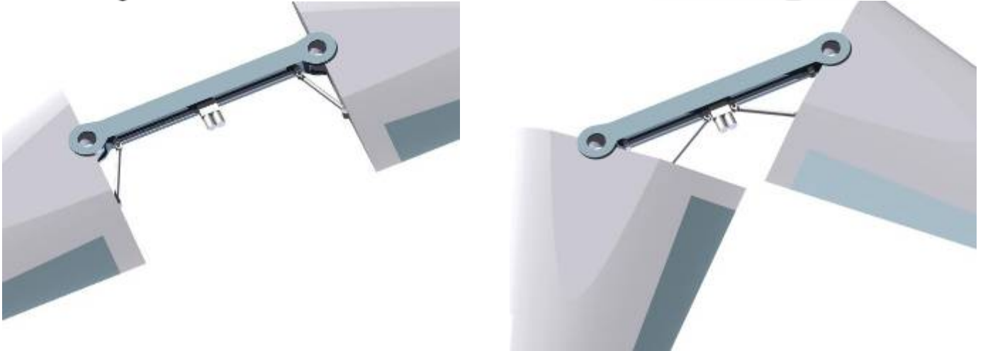
Figure 6.33: Ball actuator system as wing sweep mechanism
