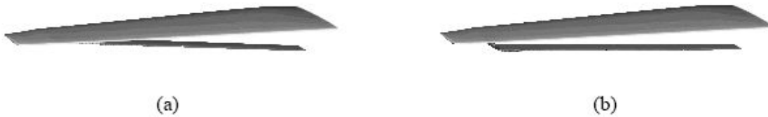
Figure 13.4 a) Intersection without arch b) Intersection with Arch (Ref. Grasmeyer, Joel M.)
