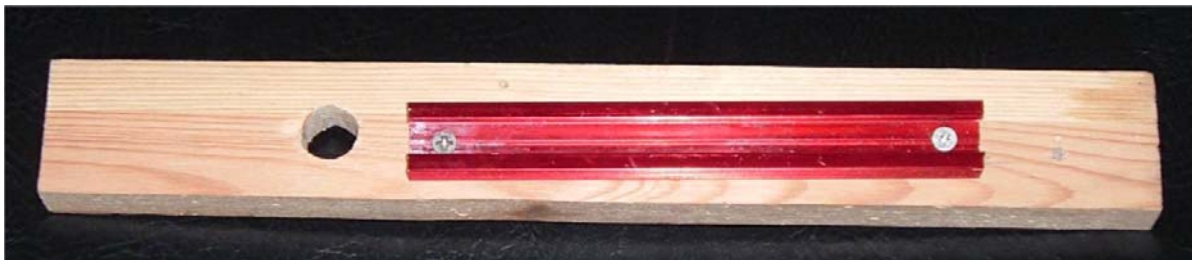
Figure 33. Image of spar mount. The aluminum track allows the rear spar to translate but keeps the rod perpendicular to the surface at all times.
