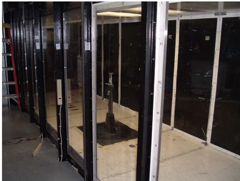
Figure 19. Image of Virginia Tech wind tunnel test section. The cross-sectional dimensions are 6' x 6'.
