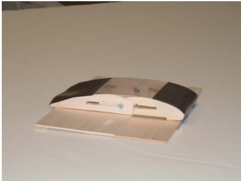
Figure 8. Model of sliding rib design. A skirt is needed to cover the gap when the chord is extended.
