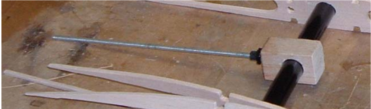
Figure 32. Image of chord block and power screw. This image was before the rear spar was installed.
