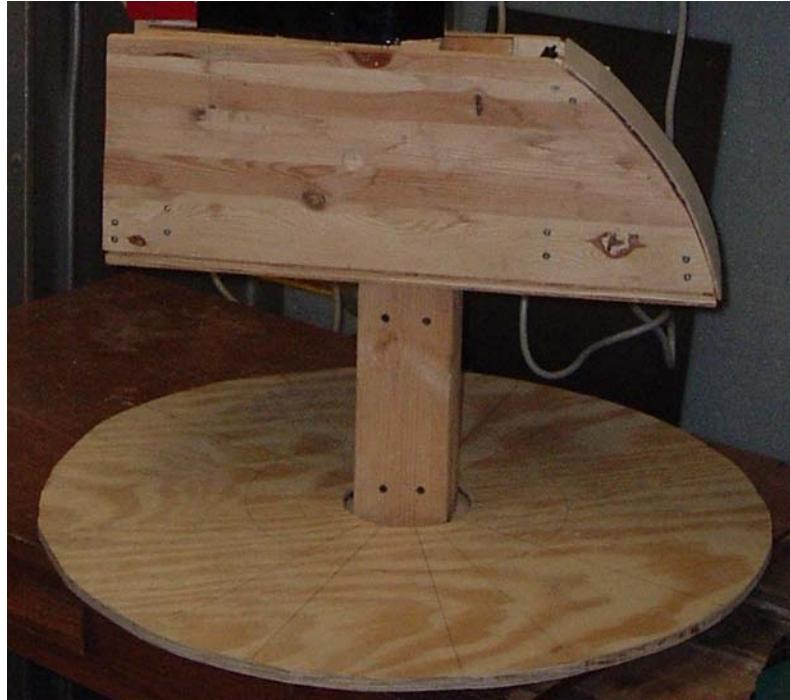
Figure 42. Image of mock fuselage attached to wind tunnel strut. Curved side of mock fuselage points into the wind.
