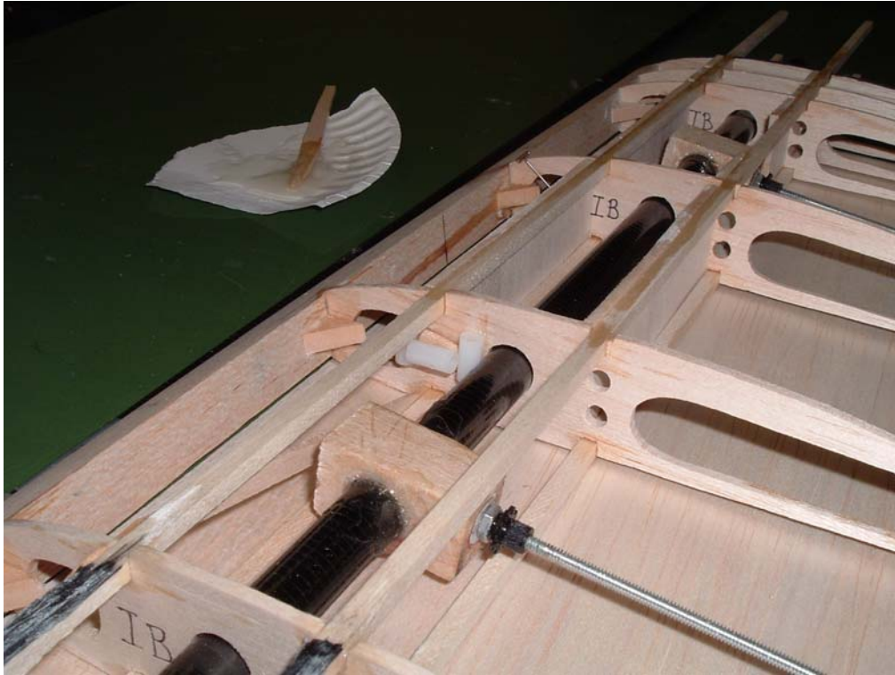
Figure 35. Image of span extension routing. To operate the span change 50 lb test fishing line was used.
