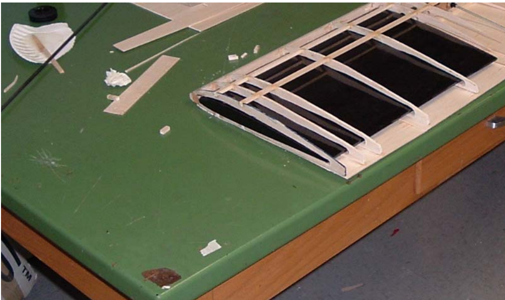
Figure 36. Image of wing with span extension in. There is no chord change where the span comes into the wing,
