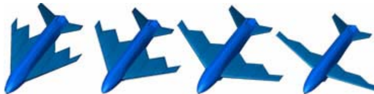
Figure 4. Image of NexGen's morphing wing concept. This design requires a stretching skin to allow the wing to morph [NewScientist.com, 2003].
