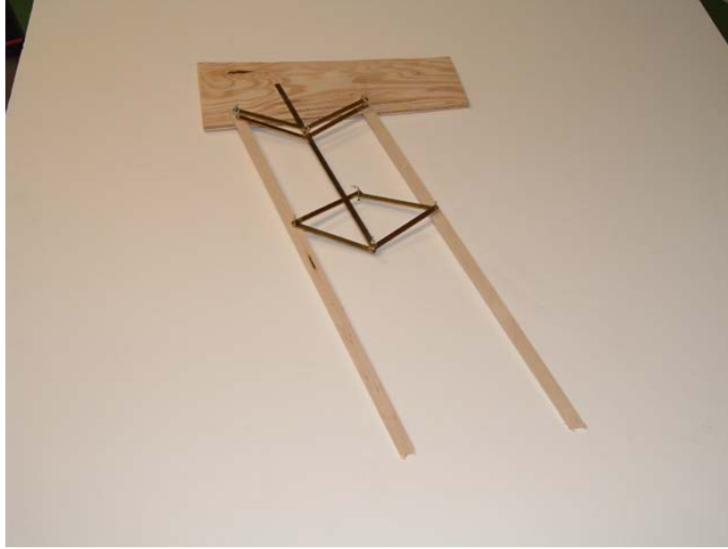
Figure 5. Model of rotating beam design. Notice diamond rod structures allow for both sweep and chord change.
