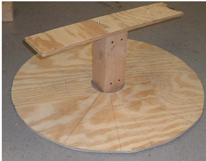
Figure 41. Image of wind tunnel test strut. Wing must be mounted to the upper surface before the base can be attached.
