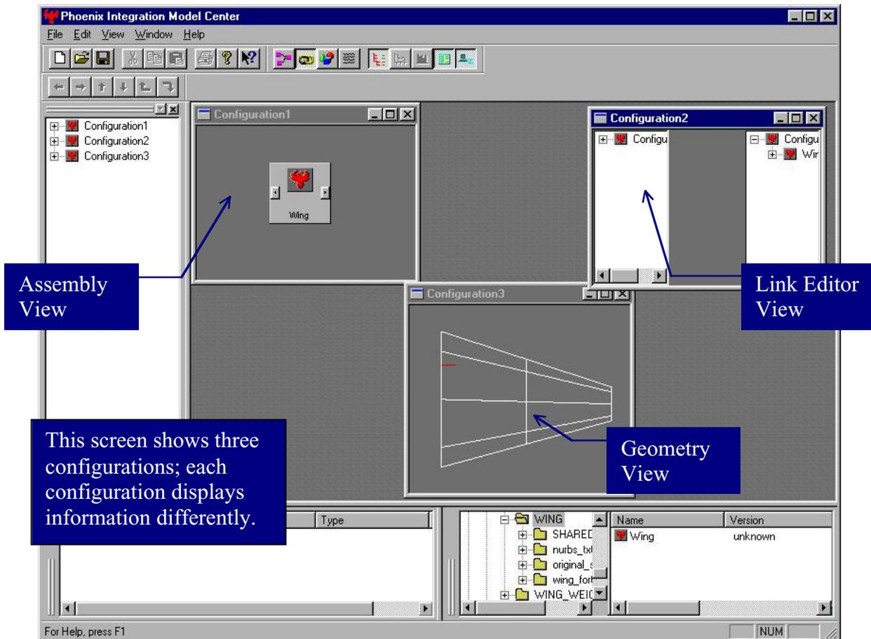
Figure 4. The ModelCenter window with three open configuration windows
