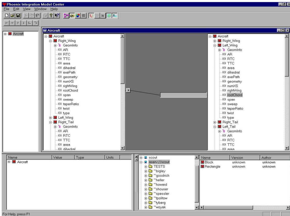
Figure 30. Link Editor showing the rootchord of the Right\_Wing linked to the Left\_Wing.
