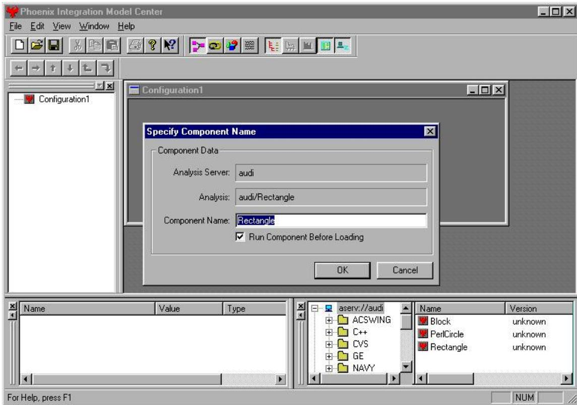
**Figure 9. When you drag components into the configuration window, you must specify a component name**
