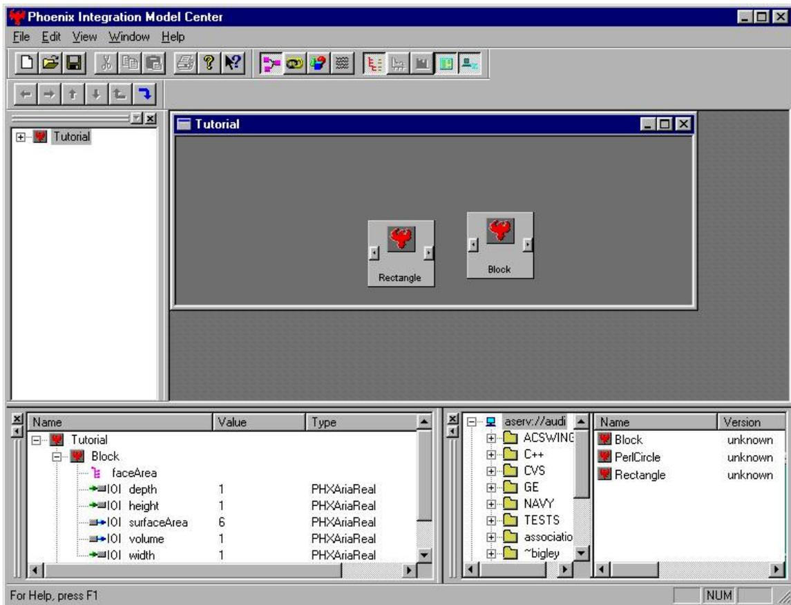
Figure 16. The ModelCenter window with a component expanded in the Data Monitor
