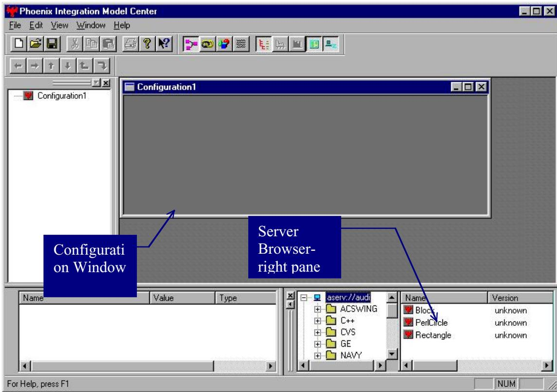
**Figure 8. The ModelCenter window displayed with one open configuration window and components in the right pane of the Server Browser**
