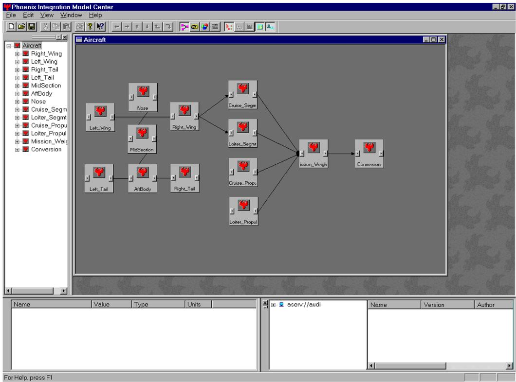
Figure 37. ModelCenter with linked components
