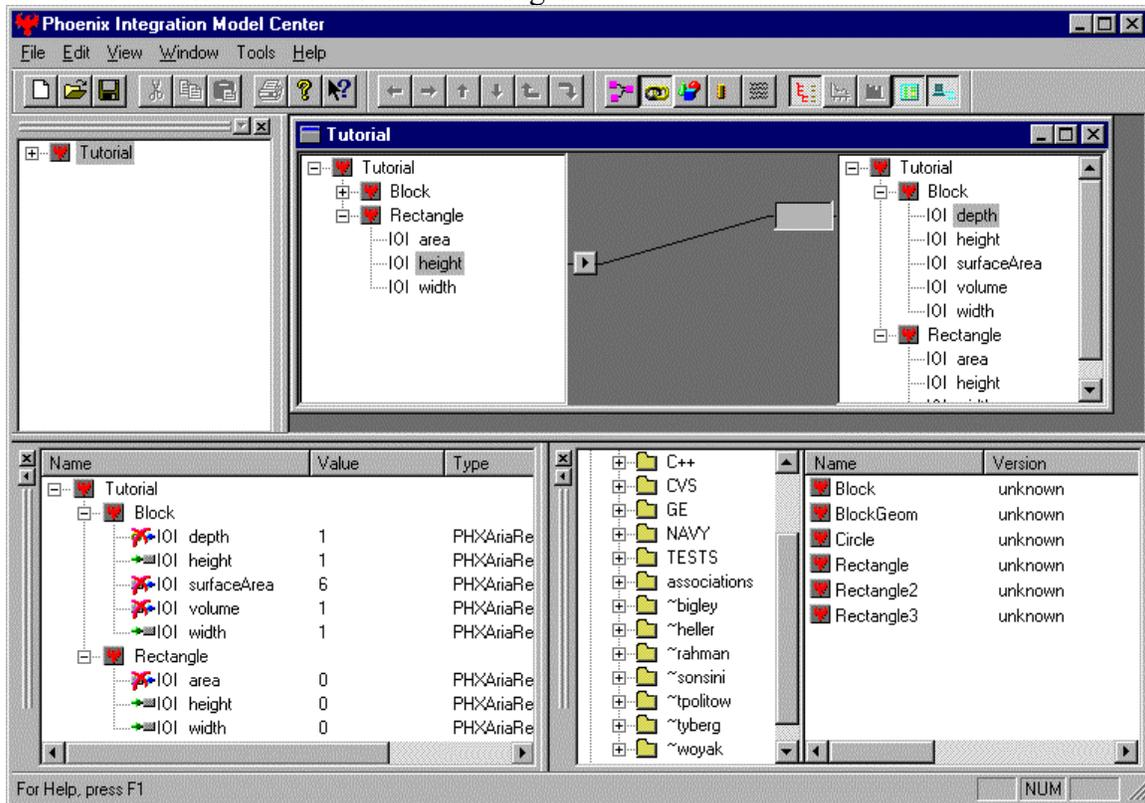
Figure 21. Two components linked in ModelCenter
