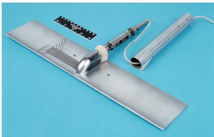
Figure 5.3c – Wing and balance block assembly, bottom view, assembled, including wind tunnel balance UT-61A and windshield
