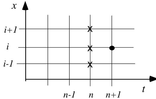
Figure 8-6. Grid points used in typical explicit calculation.
