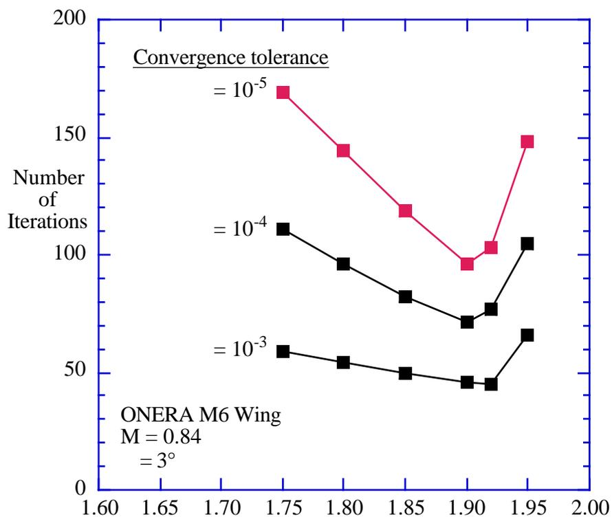
Figure 8-22. Effect of the value of  $\epsilon$  on the number of iterations required to achieve various levels of convergence.<sup>13</sup>
