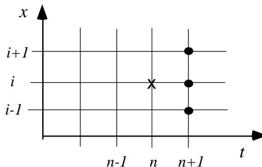
Figure 8-7. Grid points used in typical implicit calculation.
