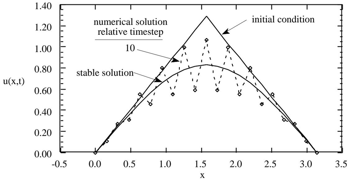
c) numerical solution using a theoretically unstable stepsize,  $\frac{t}{(\Delta x)^2} = 10$ .
