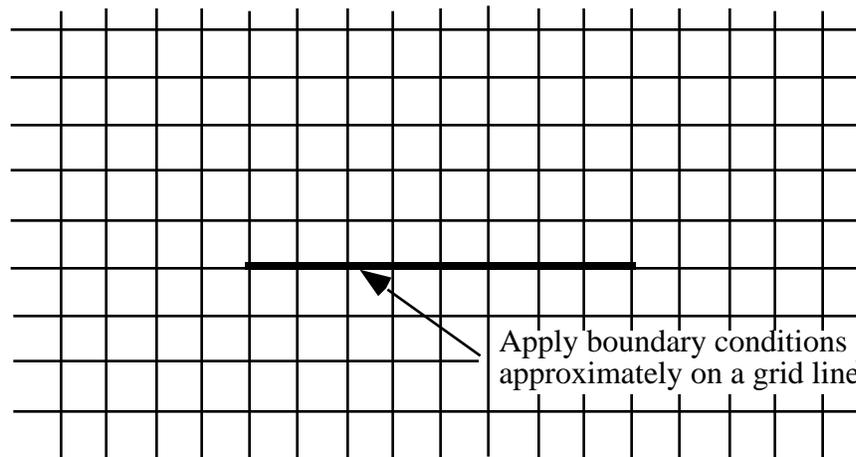
Figure 8-16. Approximate approach to boundary condition specification.
