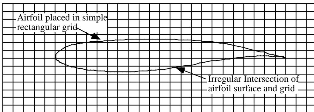
Figure 8-14. Surface passing through a general grid.
