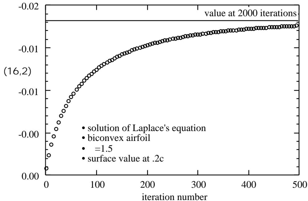
Figure 8-20. Typical variation of  $\phi$  during solution iteration.
