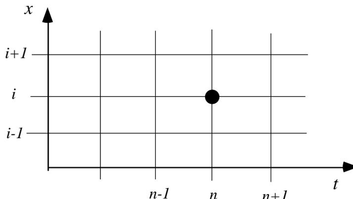
Figure 8-5. Grid nomenclature for discretization of heat equation.
