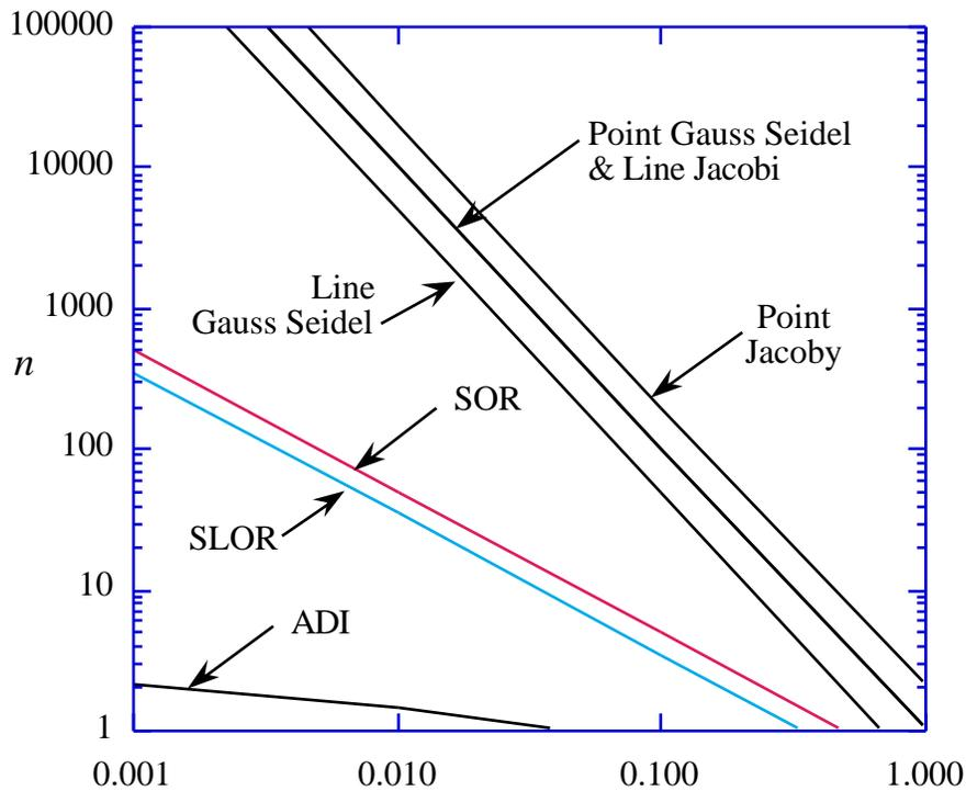
Figure 8-25. Comparison of convergence rates of various relaxation schemes (Holst<sup>10</sup>). This is the number of iterations estimated to be required to reduce the residual by one order of magnitude
