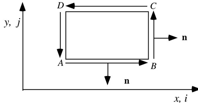
Figure 8-9. Basic nomenclature for finite volume analysis.
