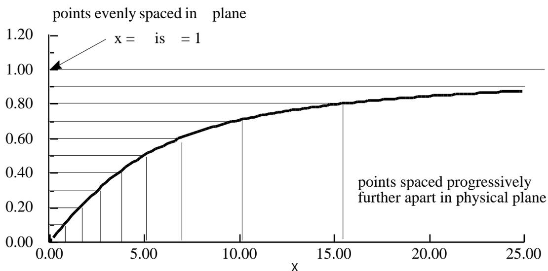
Figure 8-13. One example of a way to handle the farfield boundary condition.
