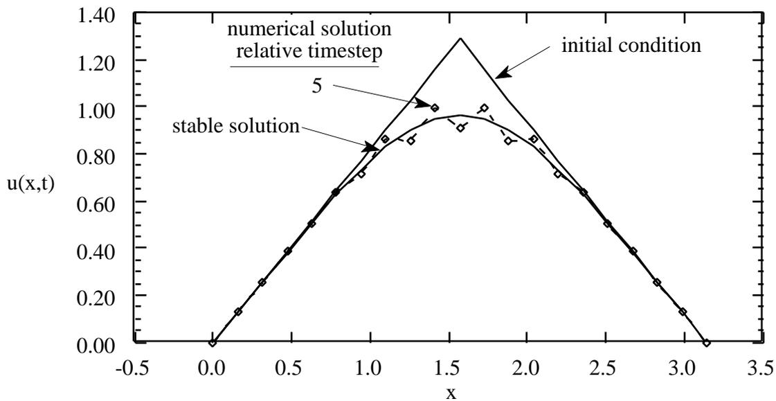
b) numerical solution using a theoretically unstable stepsize,  $\frac{t}{(\Delta x)^2} = 5$ .
