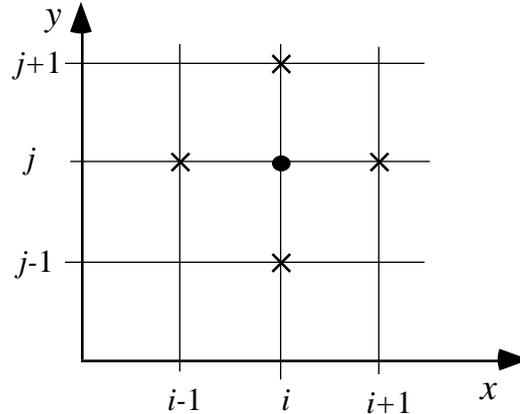
Figure 8-8. Grid points used in a typical representation of an elliptic equation.
