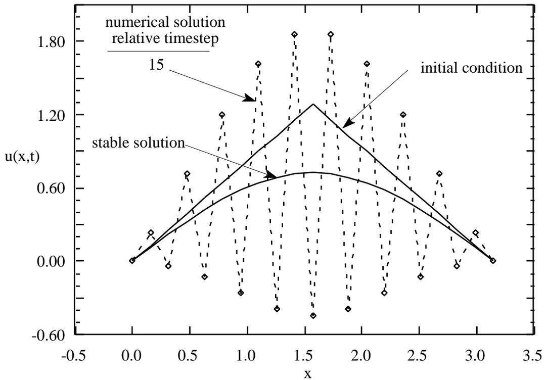
d) numerical solution using a theoretically unstable stepsize,  $\frac{t}{(\Delta x)^2} = 15$ .
