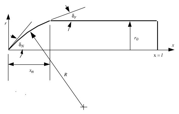
Note that the ogive is actually the arc of a circle and when  $\delta_r = 0$  the ogive ends tangent to the body, so that  $\delta_r = 0$  represents the tangent ogive body. If  $\delta_r = \delta_N$ , the cone-cylinder is recovered. If  $\delta_r = 0$  and  $\delta_N = 90^\circ$ , the spherical cap case is obtained.
