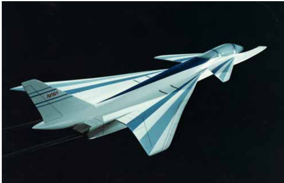
Figure 9. The Grumman Research Fighter Configuration (RFC), a joint program with NASA Langley, it had its own problems. The NTF model cost $600K and was never tested!
