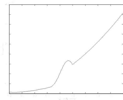
This is not a representative drag curve! It is unlikely that the drag will decrease with increased speed in this part of the drag curve. Once the speed passes the initial drag rise Mach number, the drag rate of increase may decrease, but not the drag!
