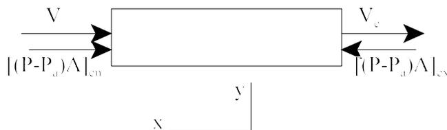
Here the pressure is indicated as  $P - P_a$ , where  $P_a$  is the atmospheric pressure, because the atmospheric pressure acts on the entire control volume, and only the difference from that pressure contributes to the unbalance force.
