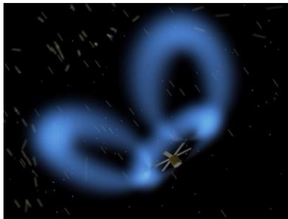
Figure 2.21: Magnetic Solar Sail. 18
