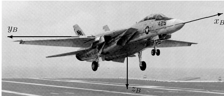
Figure 2.4: Body-Axis Reference Frame. x_B and z_B are in the aircraft plane of symmetry.
