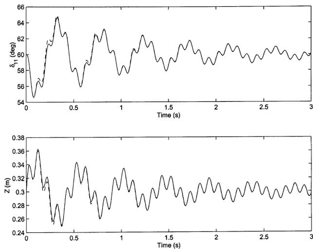
Fig. 6. Initial conditions response for  $P = 2500$ : nonlinear (---) and linear models (—).
