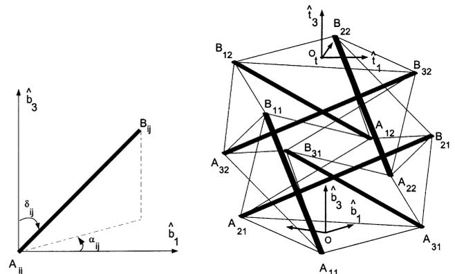
Fig. 2. Two stage SVD tensegrity structure.
