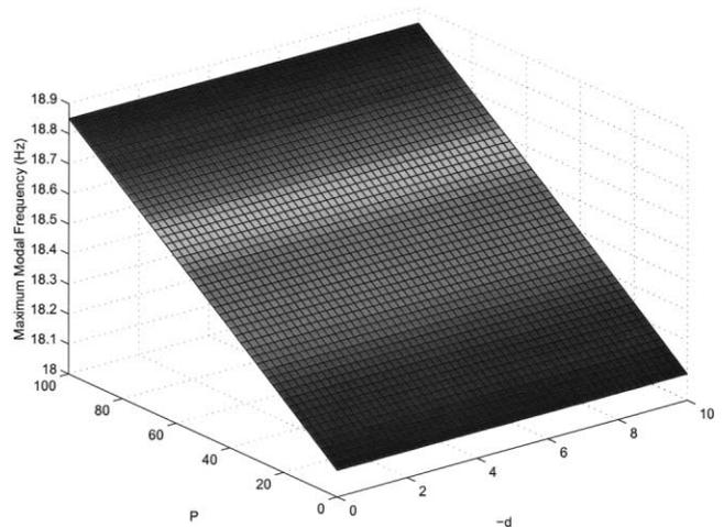
Fig. 18. Maximum modal frequency for two stage SVDT.
