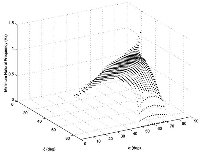
Fig. 13. Minimum natural frequency for two stage SVDT.
