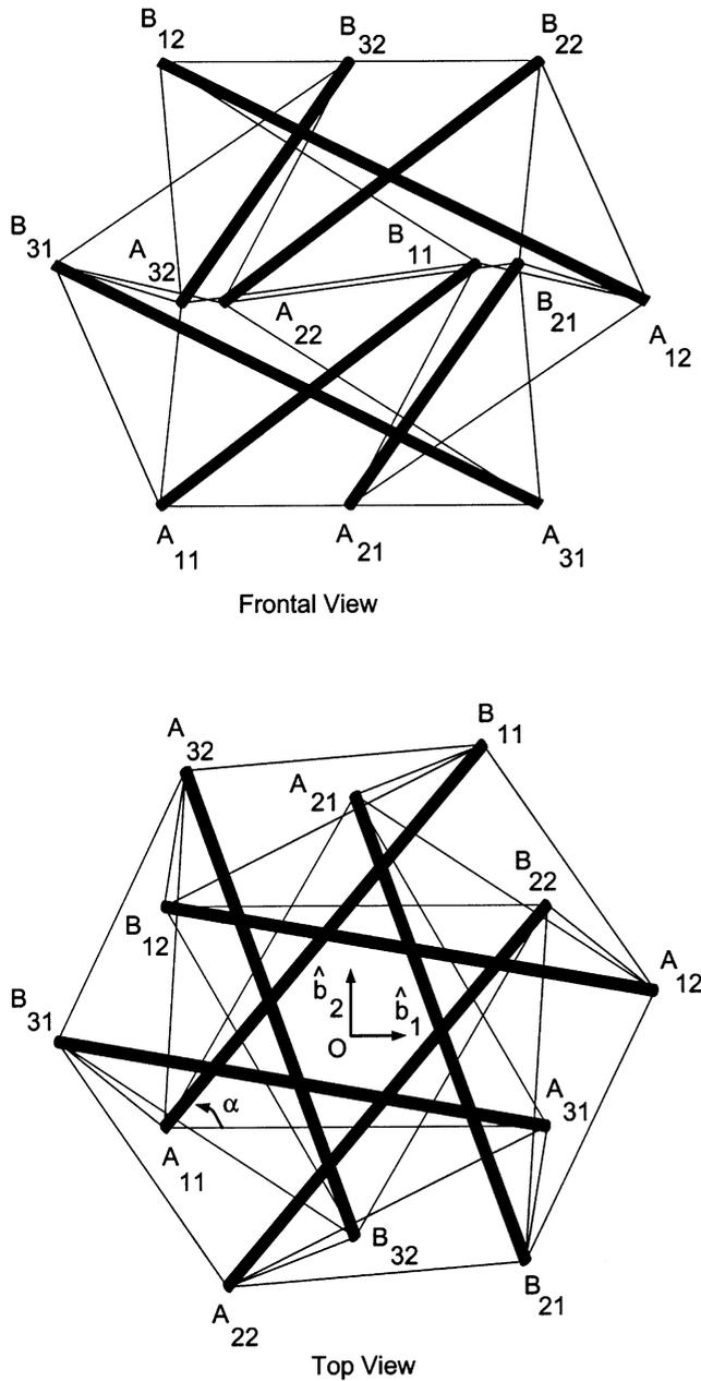
Fig. 3. Symmetrical prestressable configuration.
