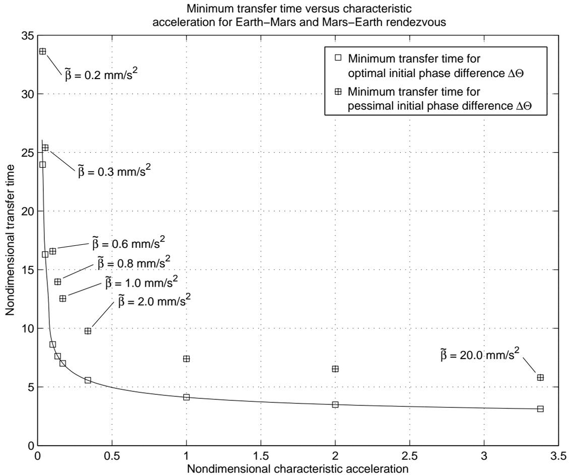
Figure 10. Minimum transfer time for optimal and pessimal initial phase difference between Mars and Earth.
