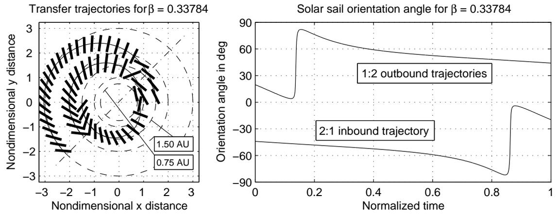
Figure 4. Minimum-time orbit transfer system symmetry.
