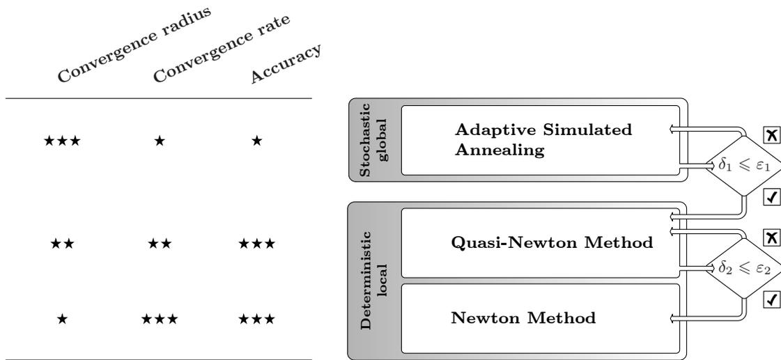
Figure 2. Cascaded numerical algorithm for solving the optimal control problem.
