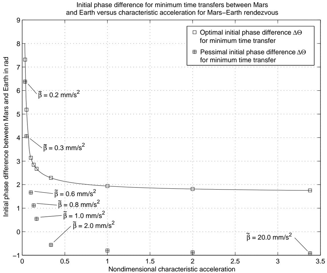
Figure 11. Optimal and pessimal initial phase difference between Mars and Earth versus characteristic acceleration.
