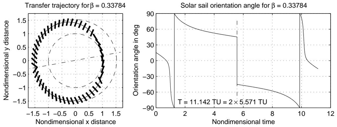
Figure 5. Earth–Mars–Earth minimum–time orbit transfer for  $\beta = 0.33784$ .
