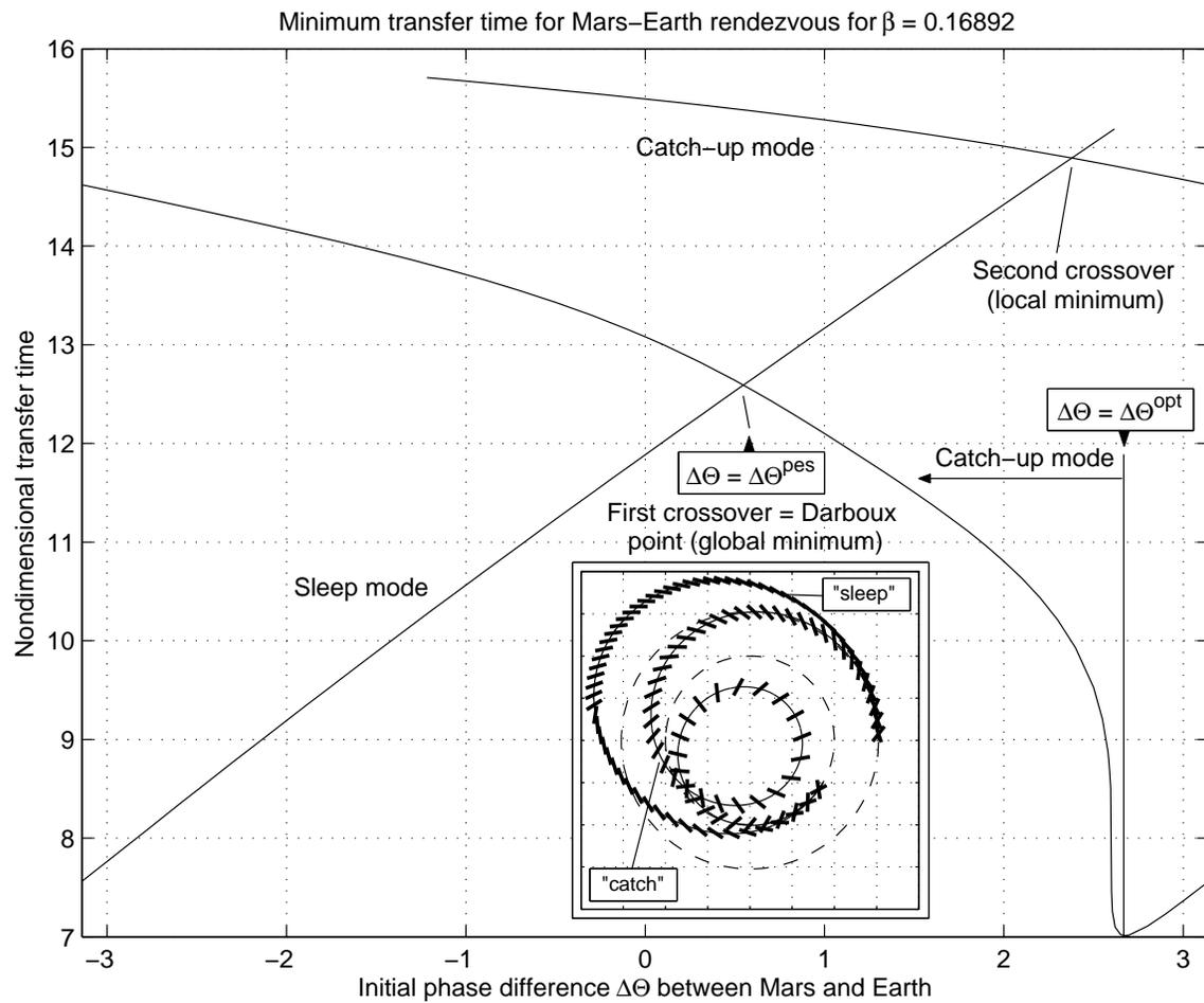
Figure 7. Minimum transfer time for Mars–Earth rendezvous for  $\beta = 0.16892$ .
