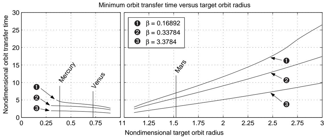
Figure 3. Transfer time as a function of target orbit radius. Initial orbit radius is 1 AU.
