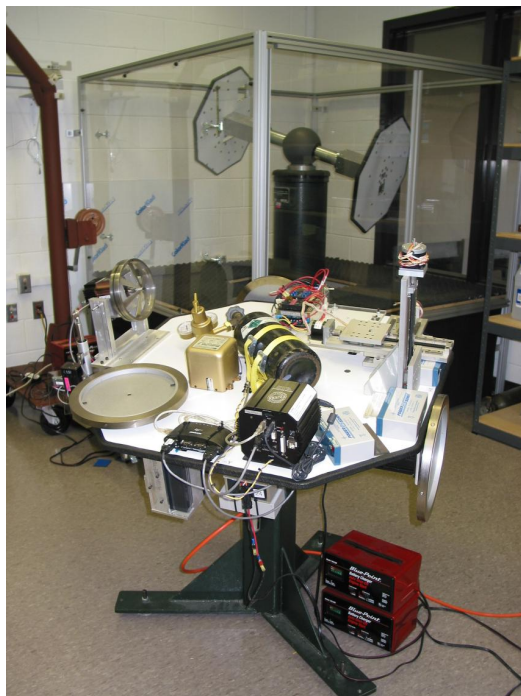
Figure 1: Virginia Tech's Distributed Spacecraft Attitude Control System Simulator
