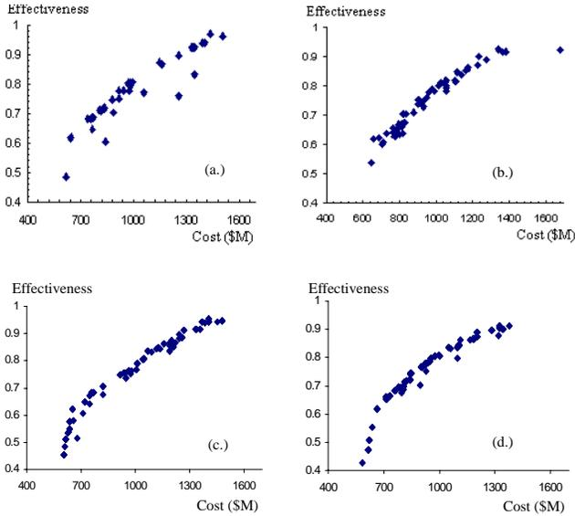
**Figure 8.** Comparison of non-dominated frontiers with different niche box sizes. (a) niche box 20 x 0.02. (b) niche box 10 x 0.01. (c) niche box 5 x 0.005. (d) niche box 2.5 x 0.0025.
