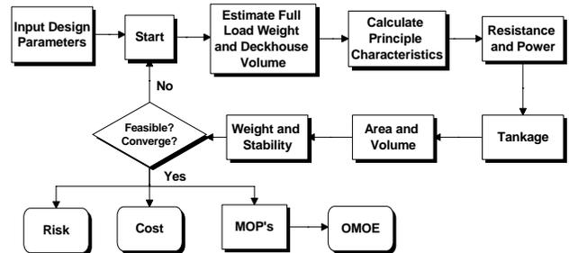
Figure 6. Ship Synthesis Model
