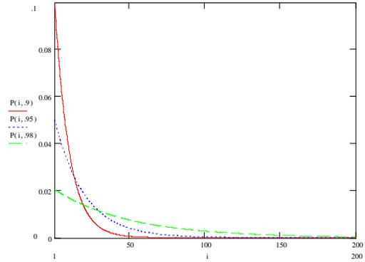
**Figure 9.** Effect of varying selection pressure on selection probability
