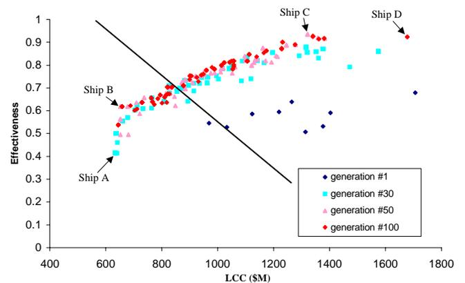
**Figure 11. N-D Frontier for DDGx (feasible only)**
