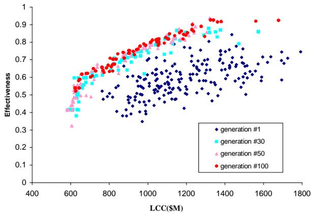
**Figure 10. N-D Frontier for DDGx with 200 individuals (feasible and infeasible)**
