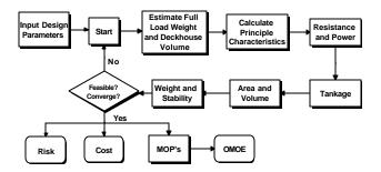
Figure 6. Ship Synthesis Model
