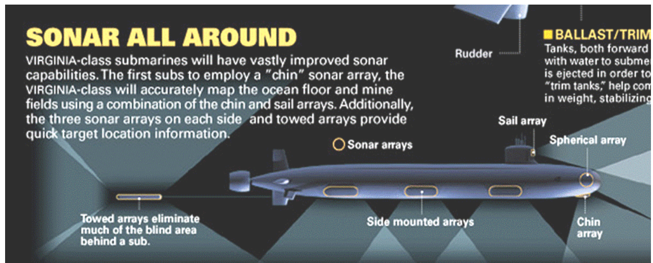
Figure 10 - Overall sonar system [navsource.org]
