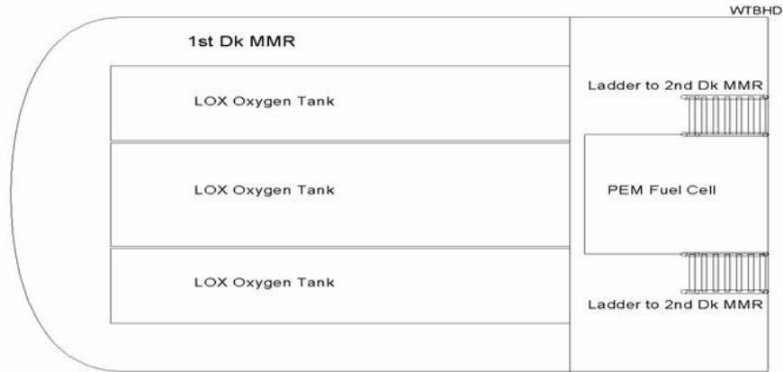
Figure 76 - MMR Deck one equipment layout
