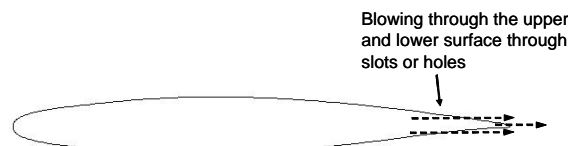
Figure 12: Concept to which the distributed-propulsion theory can be applied. Blowing through the upper and lower surface of the wing through slots or holes allows for a larger area to exhaust, hence resulting in a lower velocity and better propulsive efficiency for the same thrust.
