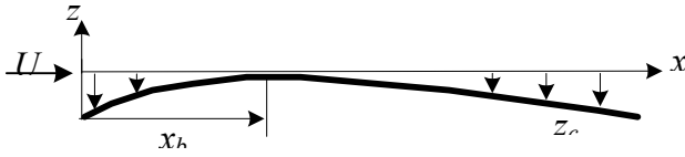
Figure 5.17: The camberline geometry for a variable camber airfoil with x_b fixed to the x-axis (Configuration B)
