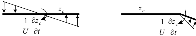
Figure 2.4: The damping terms of w ( w_d ) for a pitching airfoil and a deflecting flap
