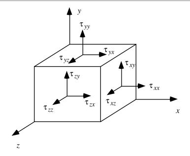
Figure 2-6. Control volume with surface forces shown.
