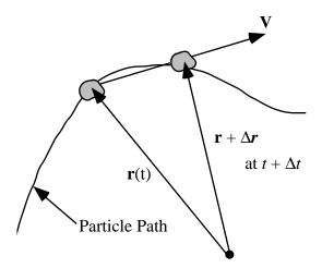
Figure 2-5. Moving particle viewed from a fixed coordinate system.
