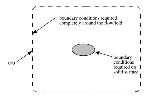
Figure 2-13. Boundary conditions required for elliptic PDEs.
