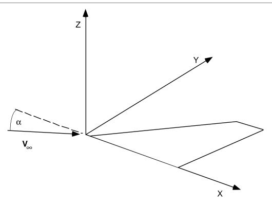
Figure 2-2 Standard coordinate system for three-dimensional flow.
