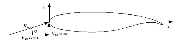
Figure 2-1 Coordinate system for two-dimensional flow.
