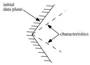
Figure 2-11. Connection between characteristics and initial condition data planes.
