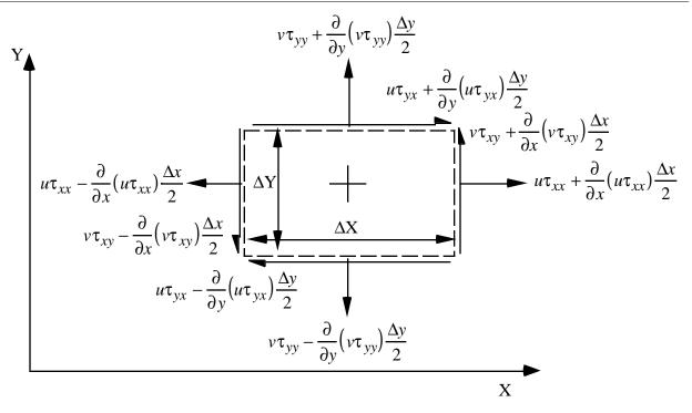
Figure 2-9 Work done on a control volume.
