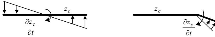
Figure 3.2. The damping terms of the boundary condition for a pitching airfoil and a deflecting flap.
