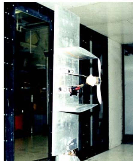
Figure 1: Inboard Winglet Model in Tunnel
