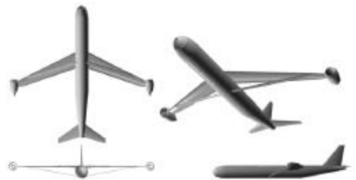
Tip mounted engine strut-braced wing design
