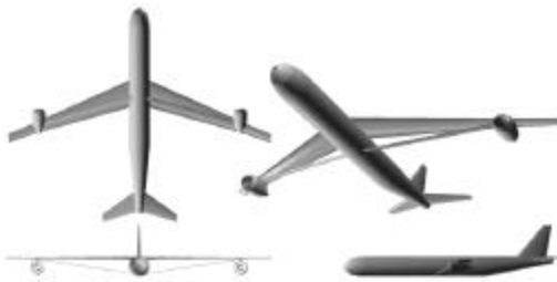
Wing mounted engine strut-braced wing design
