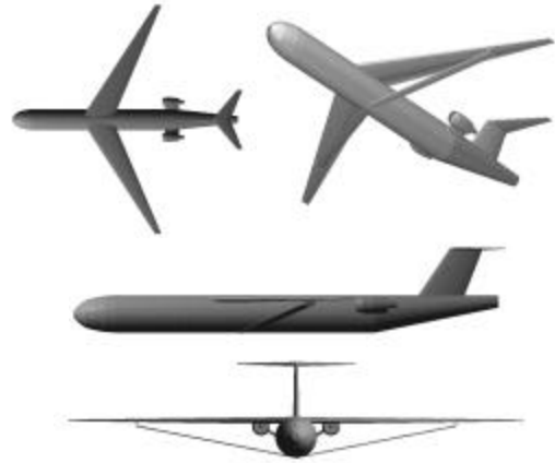
Fuselage mounted engine strut-braced wing design
