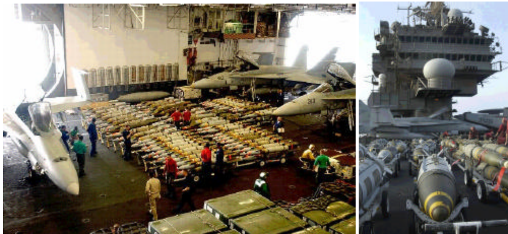
Figure 7 – Hangar Deck and Flight Deck Bomb Farms (CVN)
