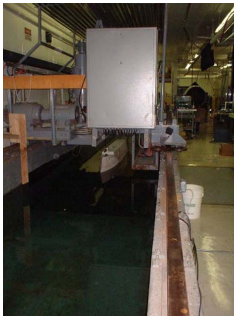
Figure 2. Tow Tank Apparatus and Model Ship
