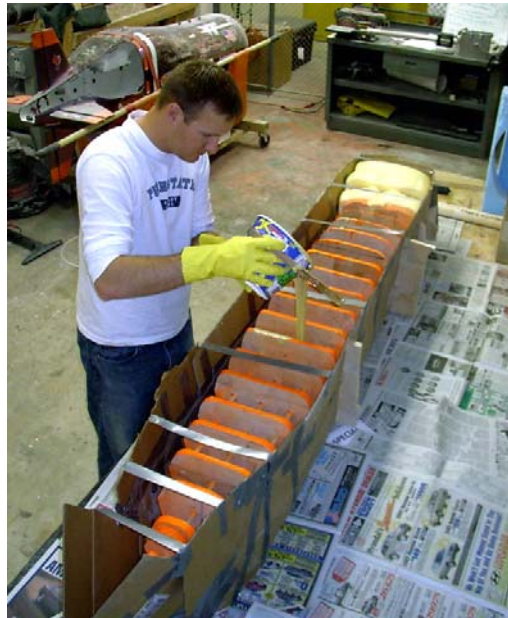
Figure 1. Foam surface being added to model frame structure
